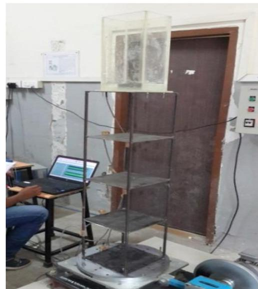
**Fig -1:** Experimental setup for tuned liquid damper
