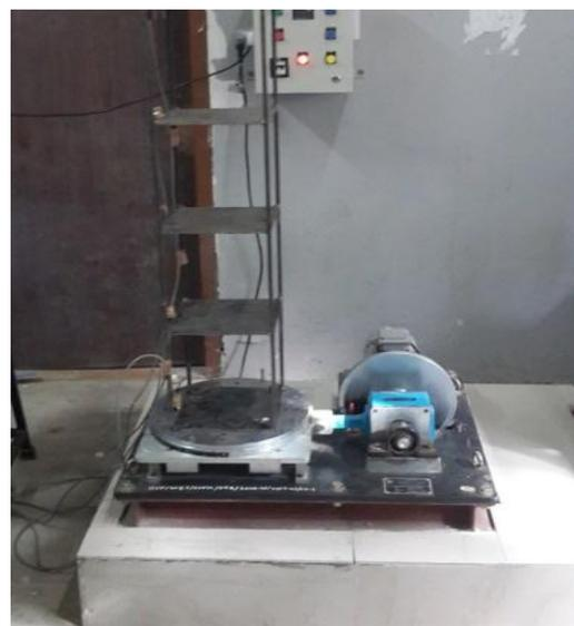
**Fig -2:** Setup without tuned liquid damper
