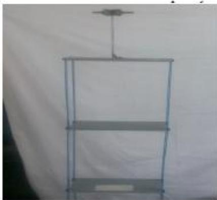
Fig -3: Structure with tuned mass damper
