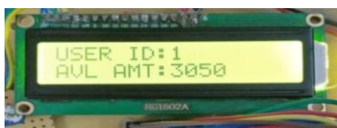
Fig -7: After fetching the data, user available amount is displayed on LCD
