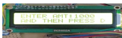
Fig -14: If recharge button is pressed, then controller ask the user to enter the recharge amount
