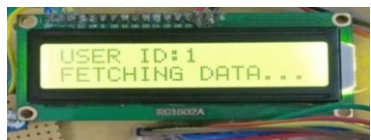
Fig -6: Controller fetching the user available amount data from the website
