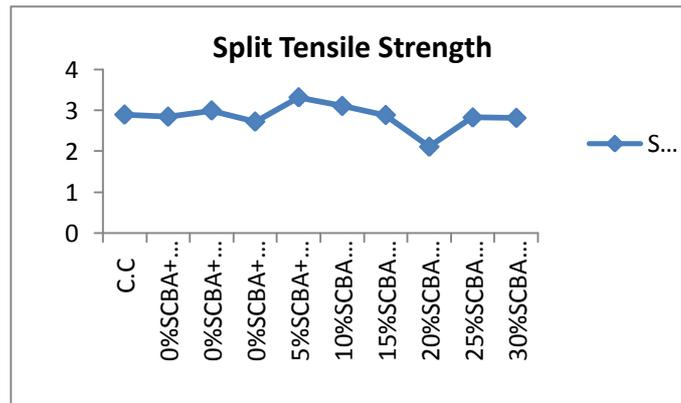
Graph 3: Showing the split tensile strength results for various SCBA & QD replacements
