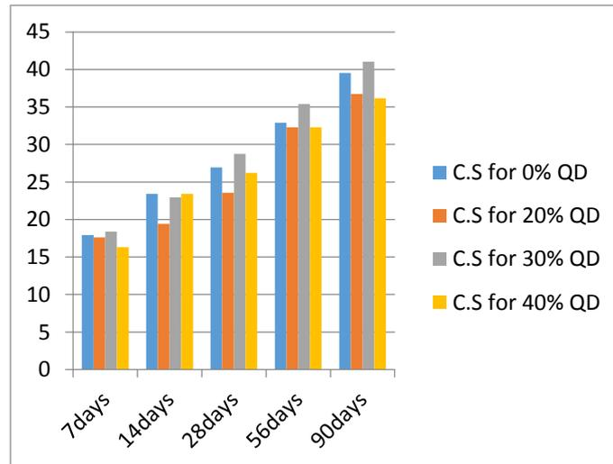
**Fig-1 Showing the comparison of compressive strength results for 0%,20% 30% & 40% QD.**
