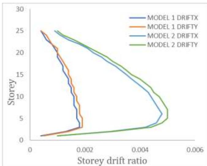
Chart -4: Storey drift ratio for M1 and M2
