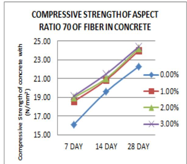
**Graph 4: Compressive Strength Of Aspect Ratio 70 Of Fiber In Concrete**
