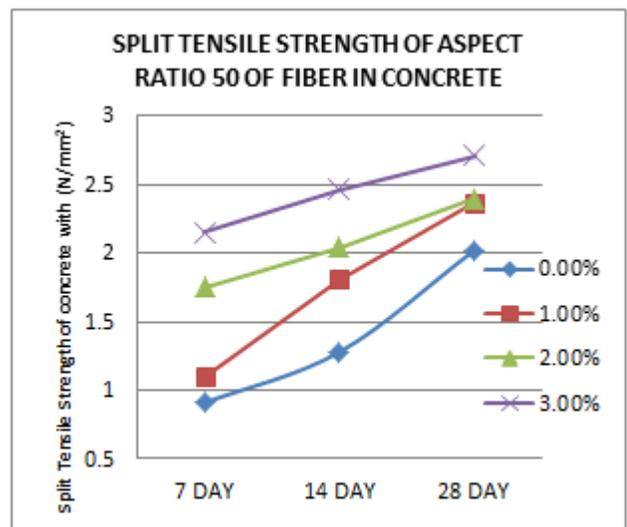
**Graph 5: Split Tensile Strength Of Aspect Ratio 50 Of Fiber In Concrete**
