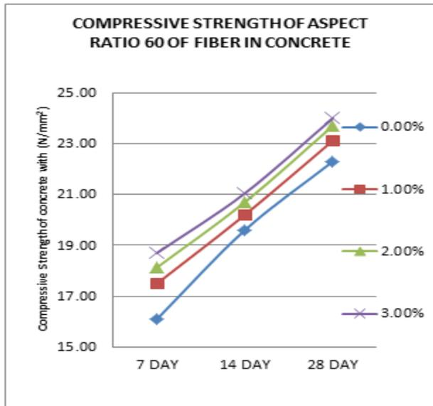
**Graph 3: Compressive Strength Of Aspect Ratio 60 Of Fiber In Concrete**
