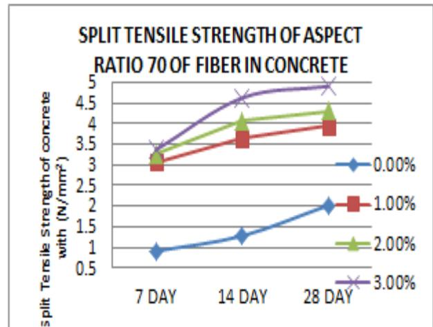
Graph 7: Split Tensile Strength Of Aspect Ratio 70 Of Fiber In Concrete
