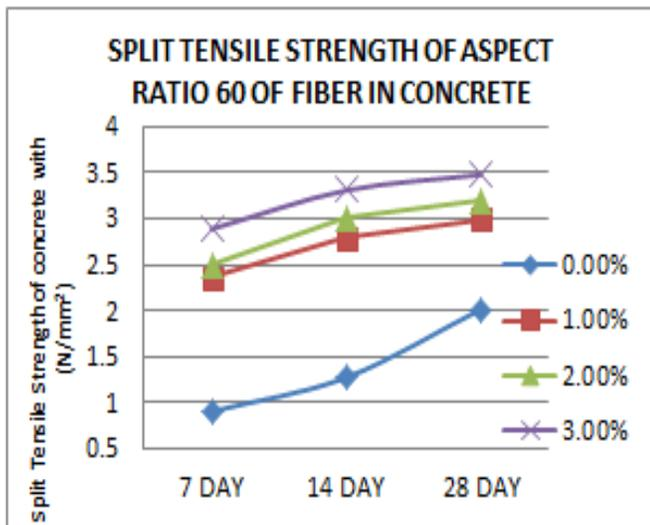
Graph 6: Split Tensile Strength Of Aspect Ratio 60 Of Fiber In Concrete
