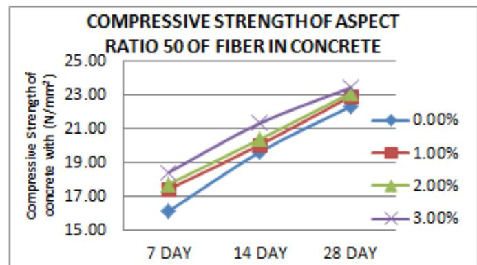
Graph 2: Compressive Strength Of Aspect Ratio 50 Of Fiber In Concrete
