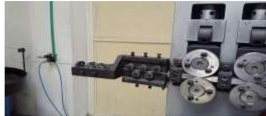
**Fig -10:** Wire Coiling Machine
