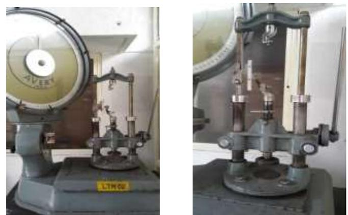
**Fig -12: Spring Testing Machine**
