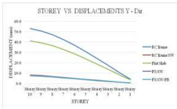
Fig -8: Storey vs. Displacements in Y-Direction
