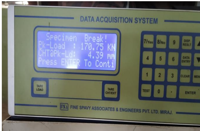
Data acquisition on UTM for deep beam
