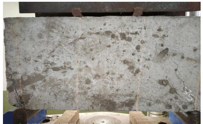
Applying a load on deep beam
