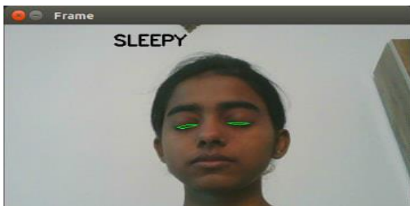
Fig. 4. Example of a successful run of drowsiness detection using reduction in vertical distance between upper and lower eyelids. The word "SLEEPY" flashed on the window of the video stream after both eyes remained closed for 4 seconds, accompanied by the sounding of an alarm.
