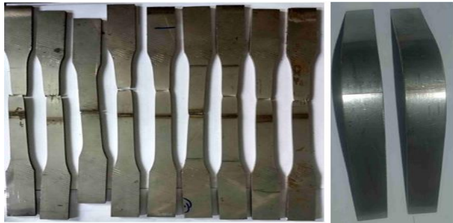
Figure 4 Tensile specimens after testing , Figure 5 Bending specimens after testing
