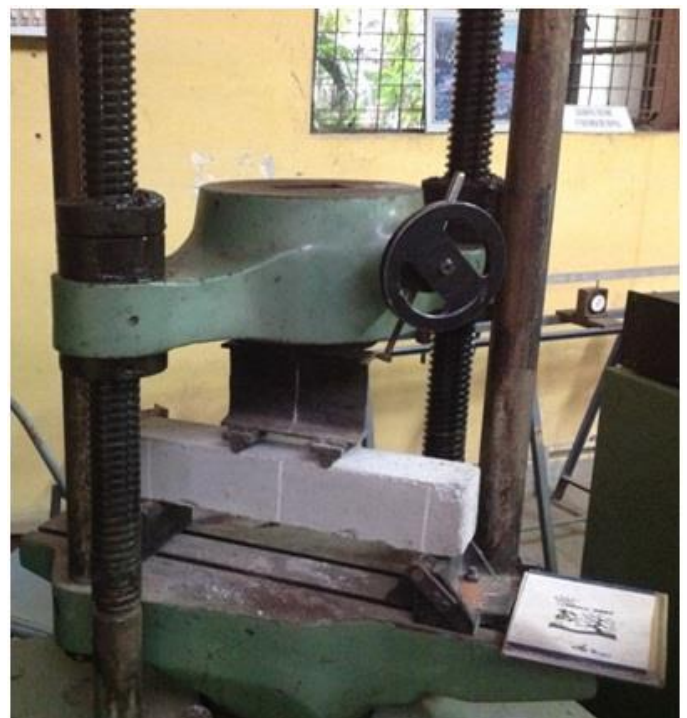
5.4.3 Experimental Setup for Flexure Test
