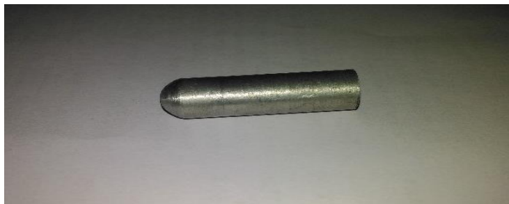
Fig. 1 Aluminum LM26 pin specimen
