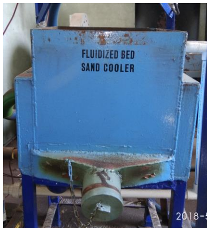
Fig.3.1 prototype of sand cooler
