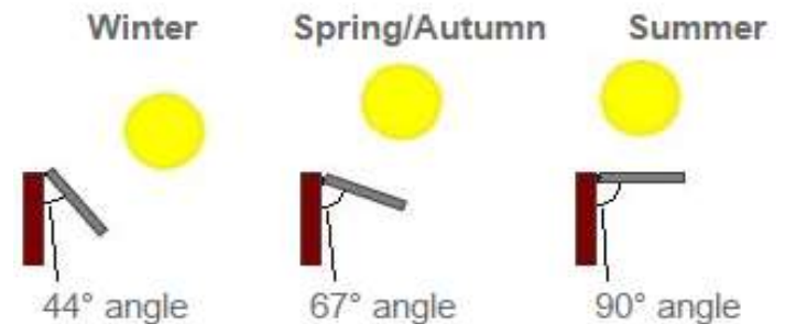
Figure 1: Average values of tilt angle for panels during different seasons for Bhopal
