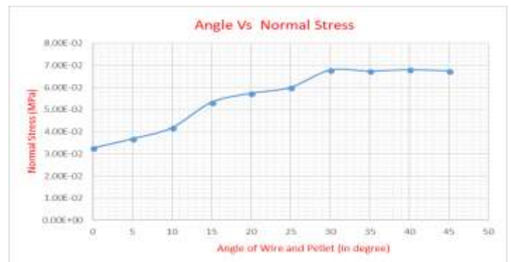
Graph no 2: Angle vs Normal Stress (X-Direction)
