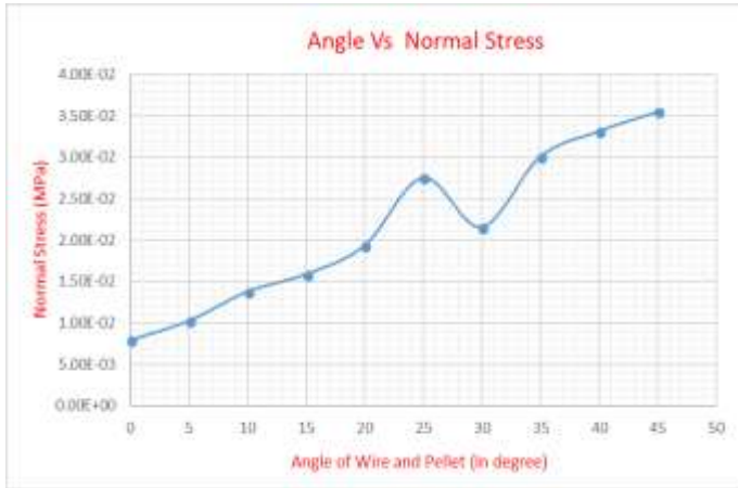
Graph no 4: Angle vs Normal Stress (Y-Direction)
