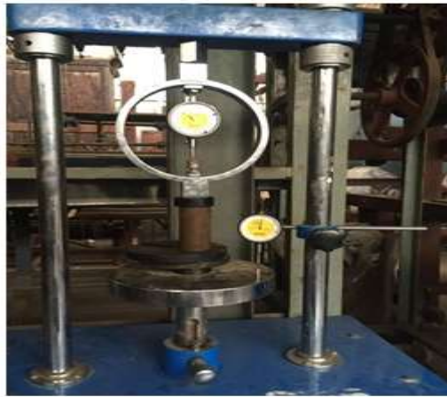
Fig -3: Unconfined strength test under process
