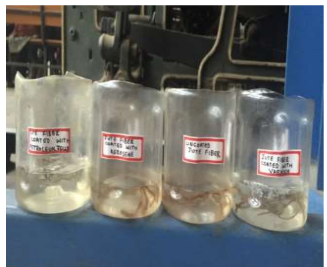
Fig -5: Water absorption test
