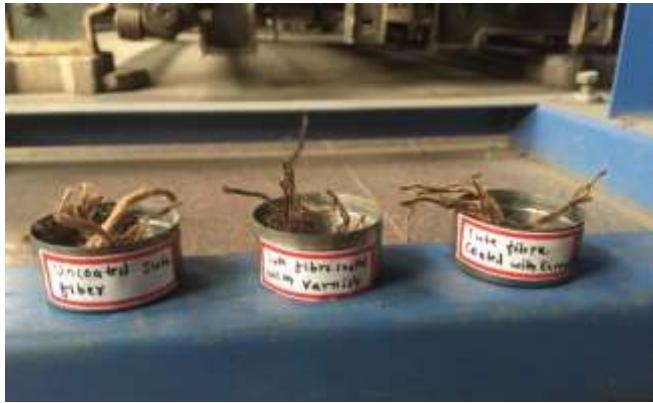
Fig -6: Jute fiber strands kept for air drying
