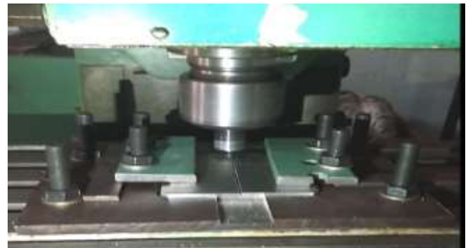
Fig -1.2: FSW process (Arrangement of workpiece and tool)
