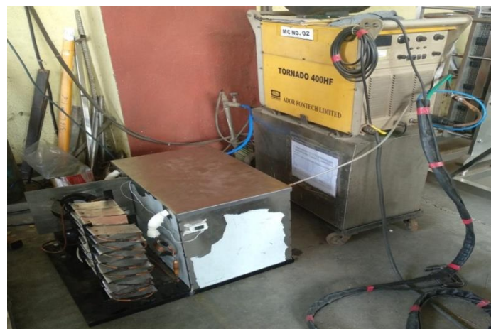
Fig.6.1. Assembly of Vapour Compression Cycle with TIG machine
