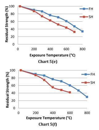
Chart 5 (a)-(f) Strength deterioration of concrete subjected to elevated temperatures for six exposure durations
