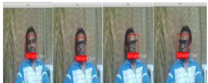
Fig - 5: Face Recognition results from different angles
