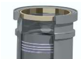
Fig -1: Cylinder with piston and cylinder liner
