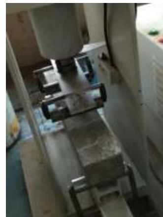
Fig -3: Flexural strength testing of beam
