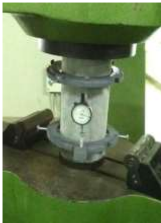
Fig -4: Modulus of elasticity testing of cylinder
