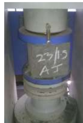
Fig -1: Compressive strength testing of cube
