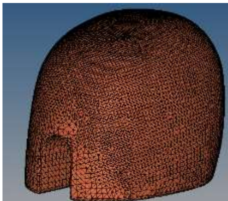
Fig-2: Detailed FE model of Headform
