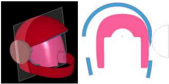
Fig-11: Cross section of helmet assembly and helmet deformation with low stiffer foam in the temporal direction
