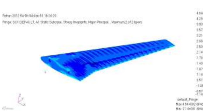
Maximum Principal Stress of meshed wing structure
