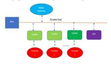
Fig1: Diagram of symmetric multi-processing system
