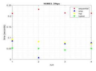
Fig8: performance analysis of sobel filter for an image size of 256px
