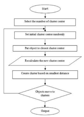
Fig6: flow chart of k-mean clustering algorithm
