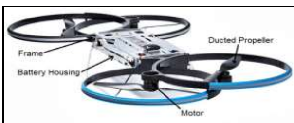
Fig-2: Simple Design of Hover Bike
