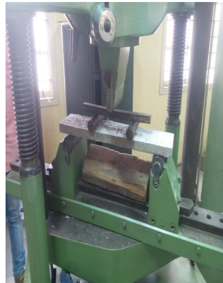
Fig - 6 Flexural strength test on ferrocement slab
