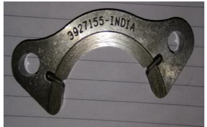
Fig- 1. Failed cam thrust plate due to wear
