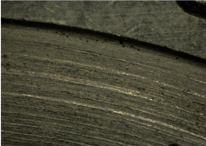
Fig -3. Wear Marks Observed At 50X
