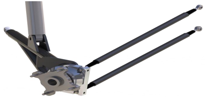
Fig -3: Semi-trailing arms with two control links
