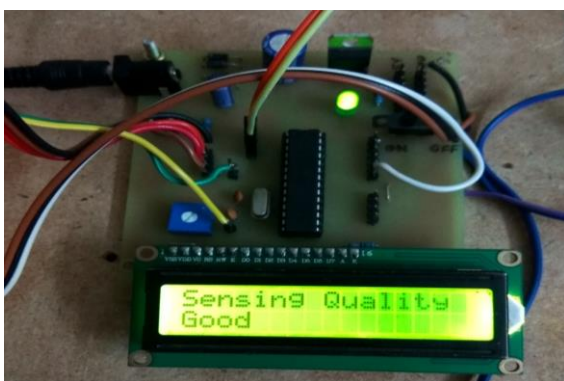
Fig -8: Fuel quality displayed on LCD after sensing fuel at inlet while filling
