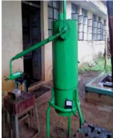
Fig 1: Pyrolysis unit to produce biodiesel
