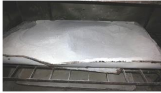
Fig -1: Fly Ash dried in oven
