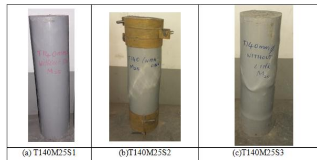
Figure 3 Typical Failure modes of 140 mm diameter specimens
