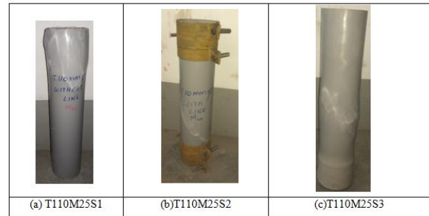
Figure 2 Typical failure mode of 110 mm diameter specimens
