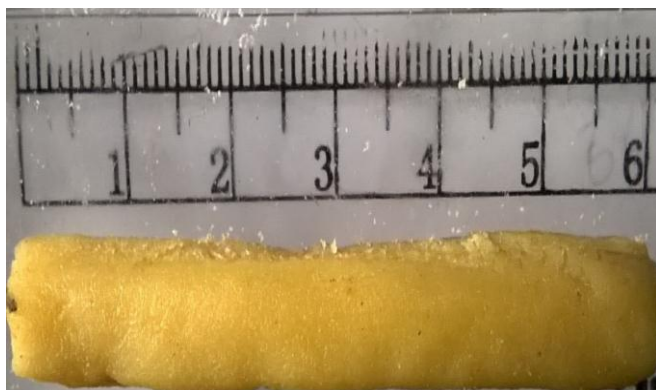
Figure 23: The pasta cut out by the 30mm chinchin cutting shaft
