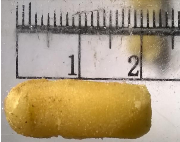
Figure 22: The pasta cut out by the 20mm chinchin cutting shaft
