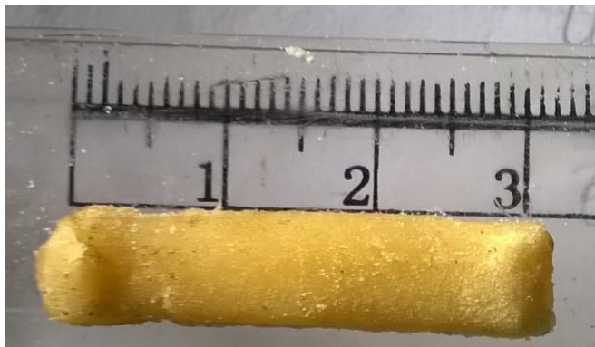
Figure 22: The pasta cut out by the 20mm chinchin cutting shaft
