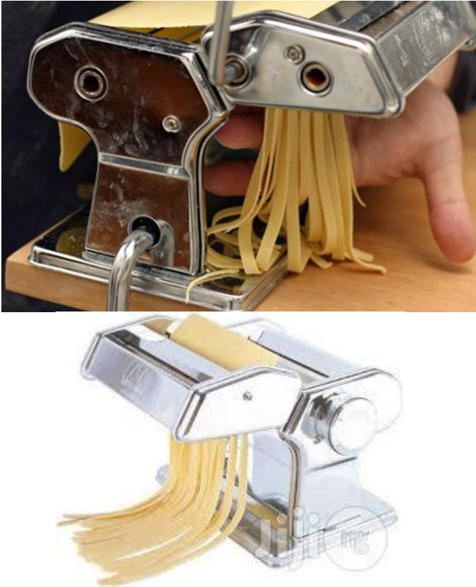
Figure 2: Existing chinchin cutting machine in operation [7]
