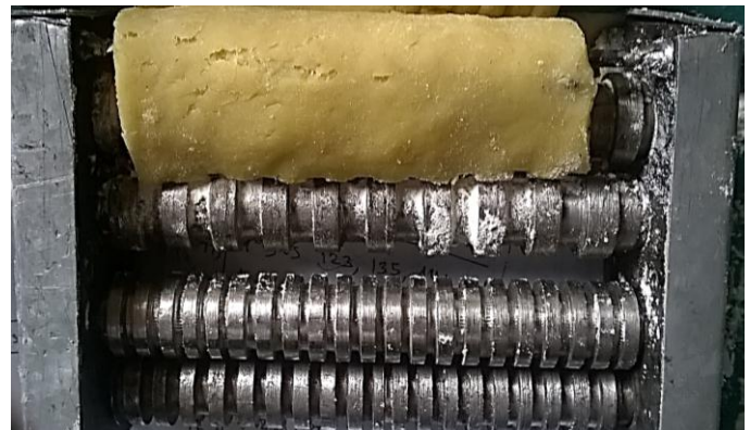
Figure 21: The fabricated prototype of the domestic chinchin cutting machine in operation
