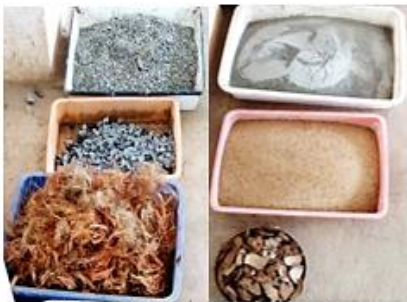
Figure 4.15: Materials for concrete mix
