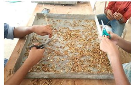
Figure 4.2: Mission grass cut for required length
