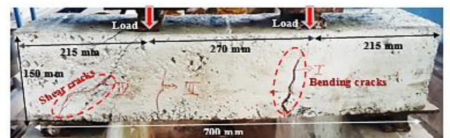
Figure 4.25: Beam specimen after flexural test
