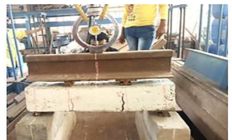
Figure 4.24: Two point load flexural test of beam specimens
