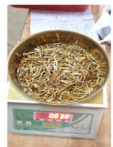
Figure 4.4: Mission grass cut for 7mm average length
