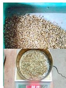
Figure 4.3: Mission grass cut for 2mm average length
