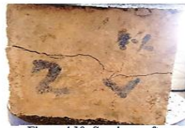
Figure 4.10: Specimen after compression test
