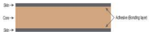
Fig -1: Foam core Sandwich
