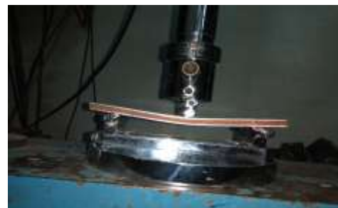
Fig -9: Mounting of Flexural specimen on UTM
