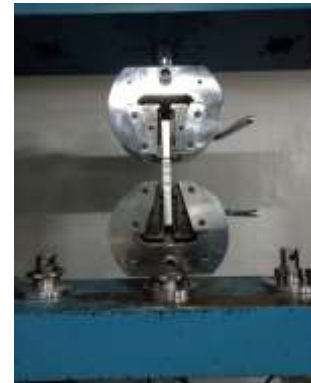
Fig -8: Mounting of tensile specimen on UTM
