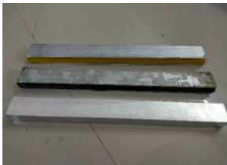
Fig -6: Specimens of Aluminium and Composite Polyurethane and polyethylene (14 mm)
