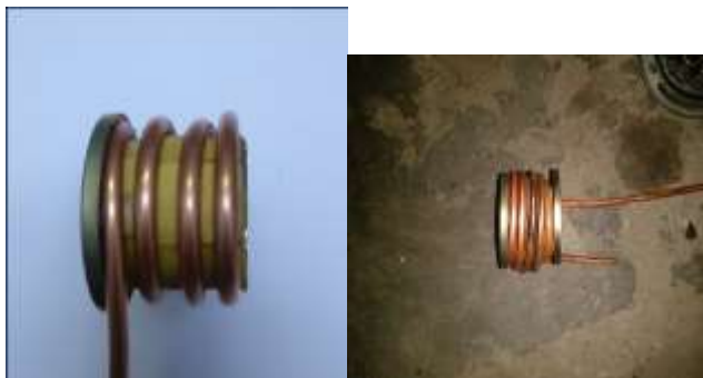
Fig-2.3: oil filter with evaporator coil
