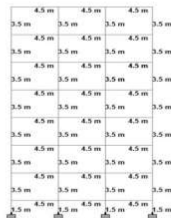
Fig -3: Elevation of building frame model
