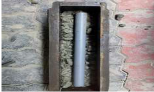
Fig 1: Beam with pipe
