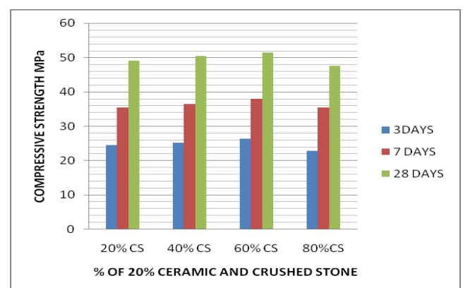
Chart - 1: Compressive strengths of 20 % of ceramic aggregate optimum and % of crushed dust.
