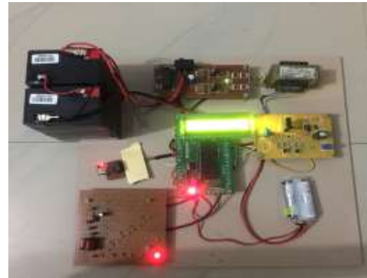
Fig -6: RF Power Harvesting Module
