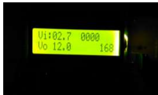
Fig -7: Input voltage and boosted output voltage
