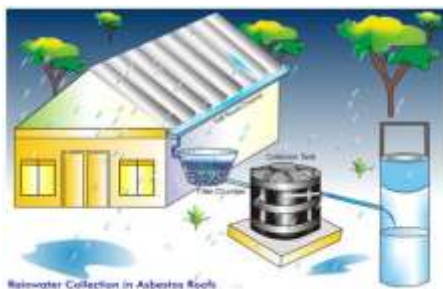
Fig. 1 Rooftop Rainwater Harvesting.
