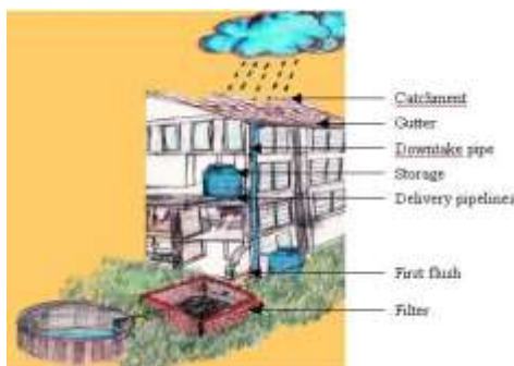
Fig. 2 Components of rooftop rainwater harvesting
