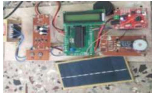
Fig- 11: experimental setup for receiver for I2V and V2V
