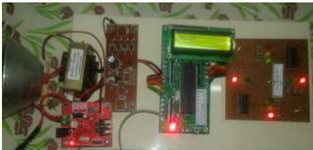
Fig-9: experimental setup for transmitter for I2V mode
