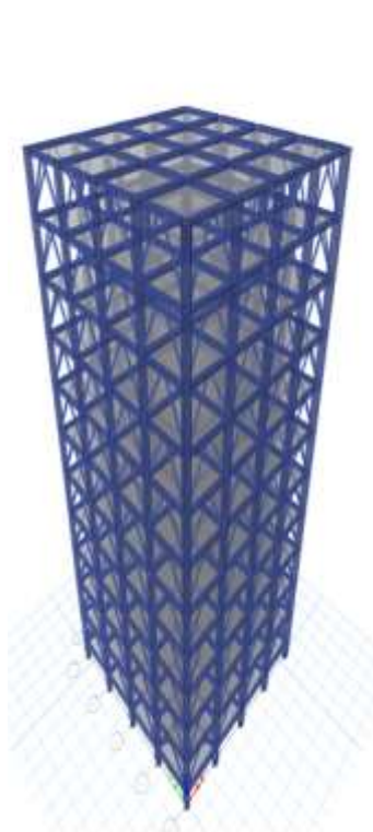
Fig -5: Model of G+10 storey building with 'V' type bracing
