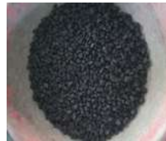
Fig-2 HDPE recycled plastic aggregates
