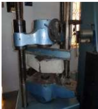
Figure-6: Flexural Strength Test
