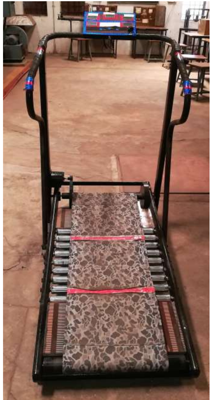
Fig-8.1 Final assembly of the manual treadmill
