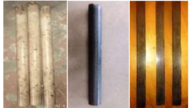
(i) Making Mold Specimen (ii) Circular Specimen for bending test (iii) Making Rectangular Specimen
