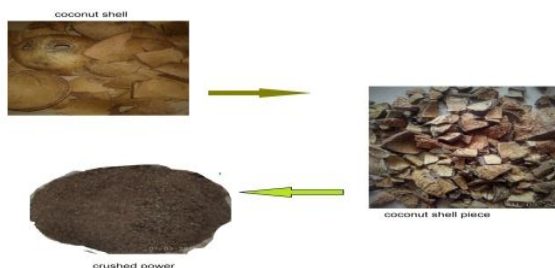
Figure.4.A. Procedure of making raw coconut shell powder
