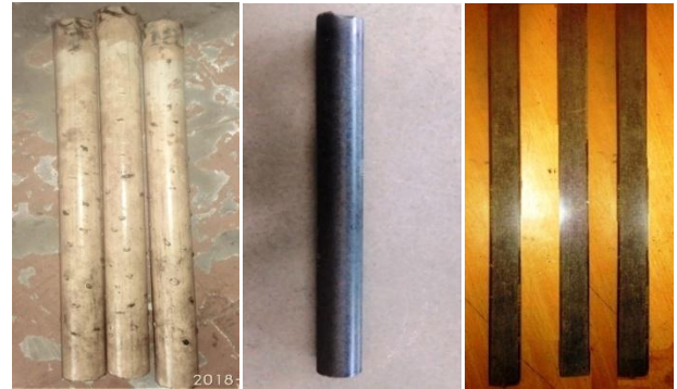
(i) Making Mold (ii) Circular Specimen (iii) Making Rectangular Specimen for bending test Specimen
